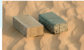
ABOVE 109 A comparison of a microbially formed BioBrick (left) and a standard concrete brick (right).
