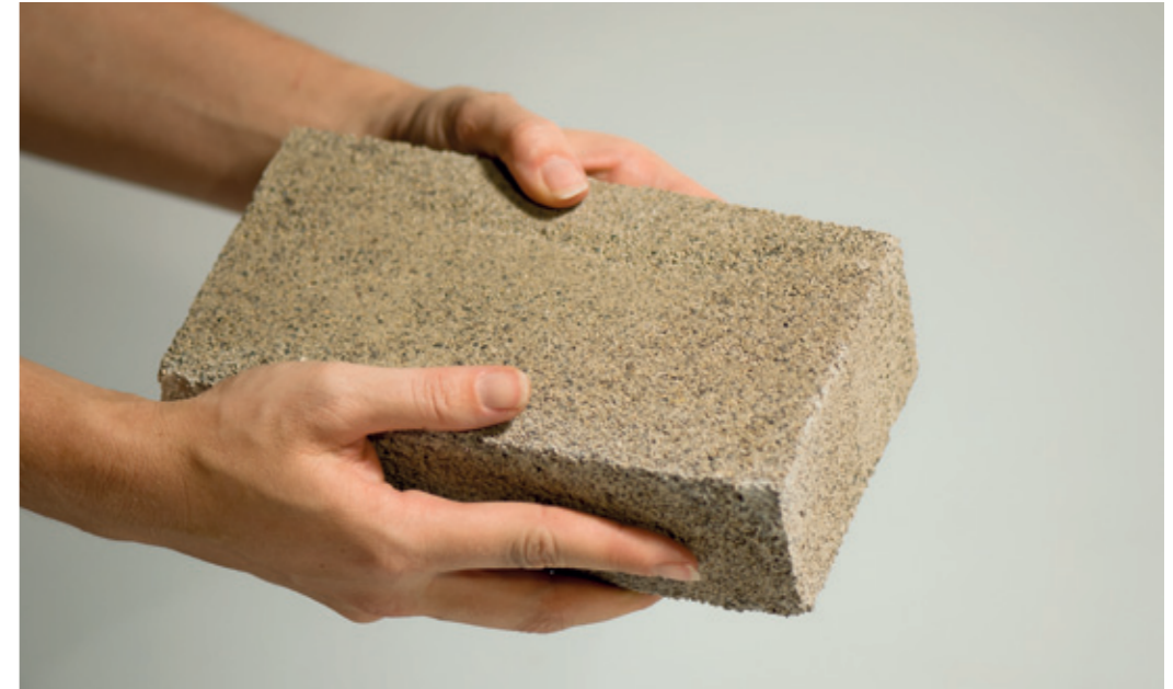
ABOVE / RIGHT 112, 113 Some 75 percent of brick production worldwide takes place in India, China, and Pakistan, where energy-intensive, traditional methods dominate. In contrast, the reactions involved in forming the BioBrick can occur at room temperature.
